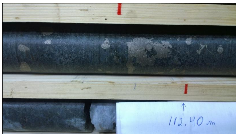
Massive Ni-Cu sulphide lumps in hole 15R312 drilled in late April 2015
