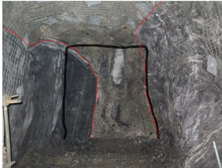
The start of the 295 SOD air-leg ore drive with face grade of 6.4% nickel
