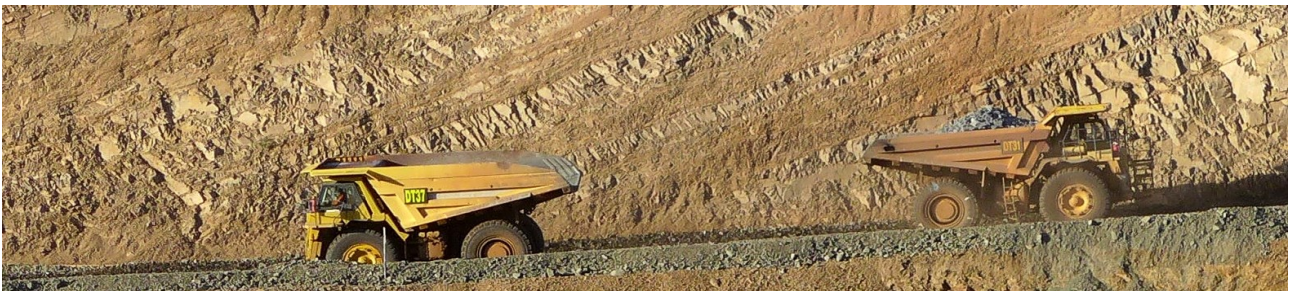
Figure 1: Haul road (ramp) into the LM2 Pit - the CuDeco mining fleet (purchased during the GFC) has performed above expectations.
