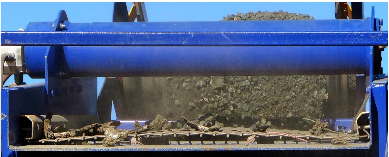
Figure 1: Scalping (recovery) of course native copper by simple crushing and screening. The native copper is flattened during cone-crushing whereas the rock breaks into smaller pieces, facilitating easy removal via appropriate screen sizing.
