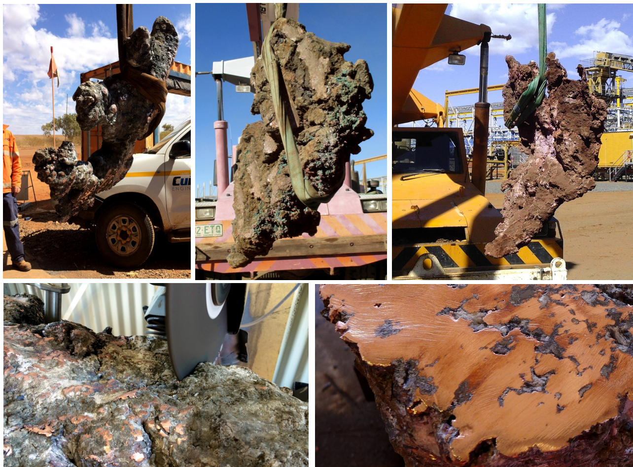
Figure 7: Masses of native copper being removed from the crushing circuit (top images) coarse native copper product averaging ~95% copper metal in concentrate at the Port of Townsville (middle) and large mass cut to reveal near solid copper metal (bottom).
