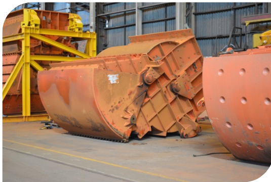
Train Load-out units being refurbished and relined.
