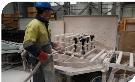
Sand Core Flow Coating (Water Based Refractory Coatings)
