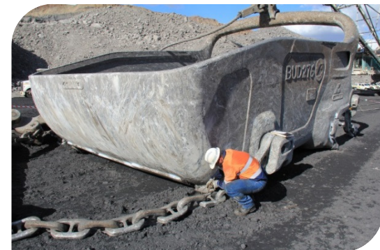
On-site inspection of Bradken Dragline bucket and Rigging Chain.
