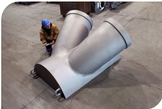
Transbay Structural Ground Level Node (11 tonne)
