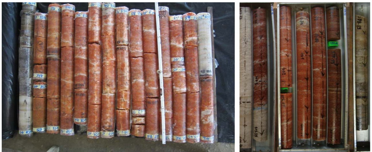
Underpinning Elementals projects is the exceptional quality potash: Left: Carnallitic intersection grading 24.65 % KCl (15.56 % K 2 O) over 11.2 metres. Right: Sylvinitic intersection grading 59.48 % KCl (37.56 % K 2 O) over 4.2 metres.
