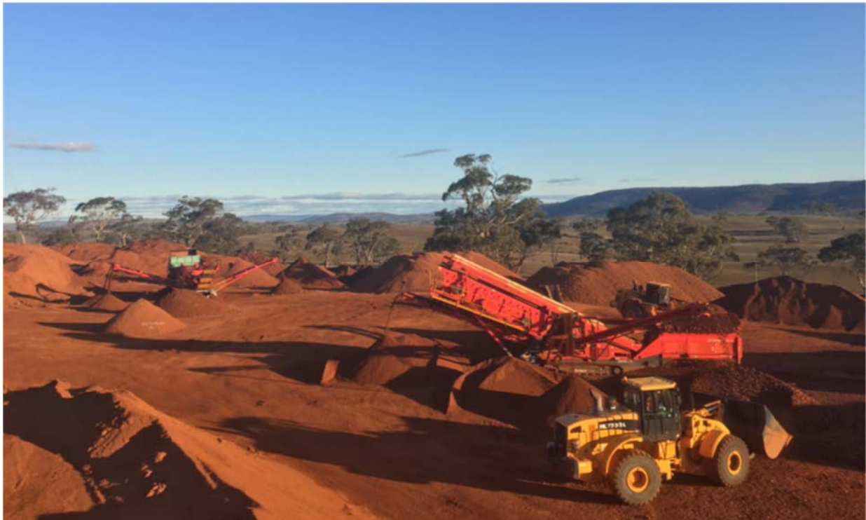
Figure 4: Bald Hill screening – simple dry screening using “Big Red” and “Li’l Red” Screening plants in tandem in Winter
