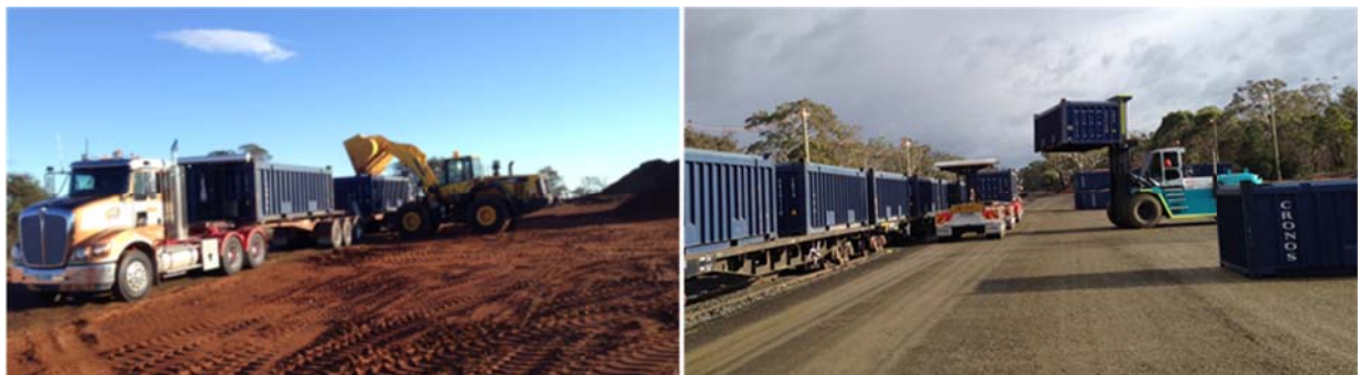
Figure 5: Bald Hill load-out – bauxite product trucked in B-double loads to Conara rail siding by TasRail
