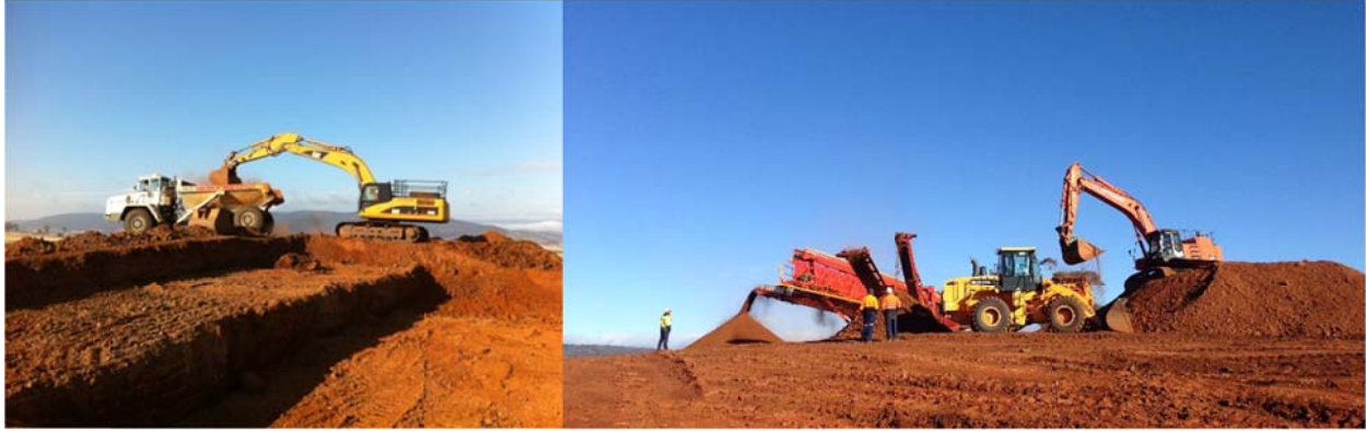
Figure 3: Bald Hill mining – simple free-dig benching, stockpiling and feeding to screens
