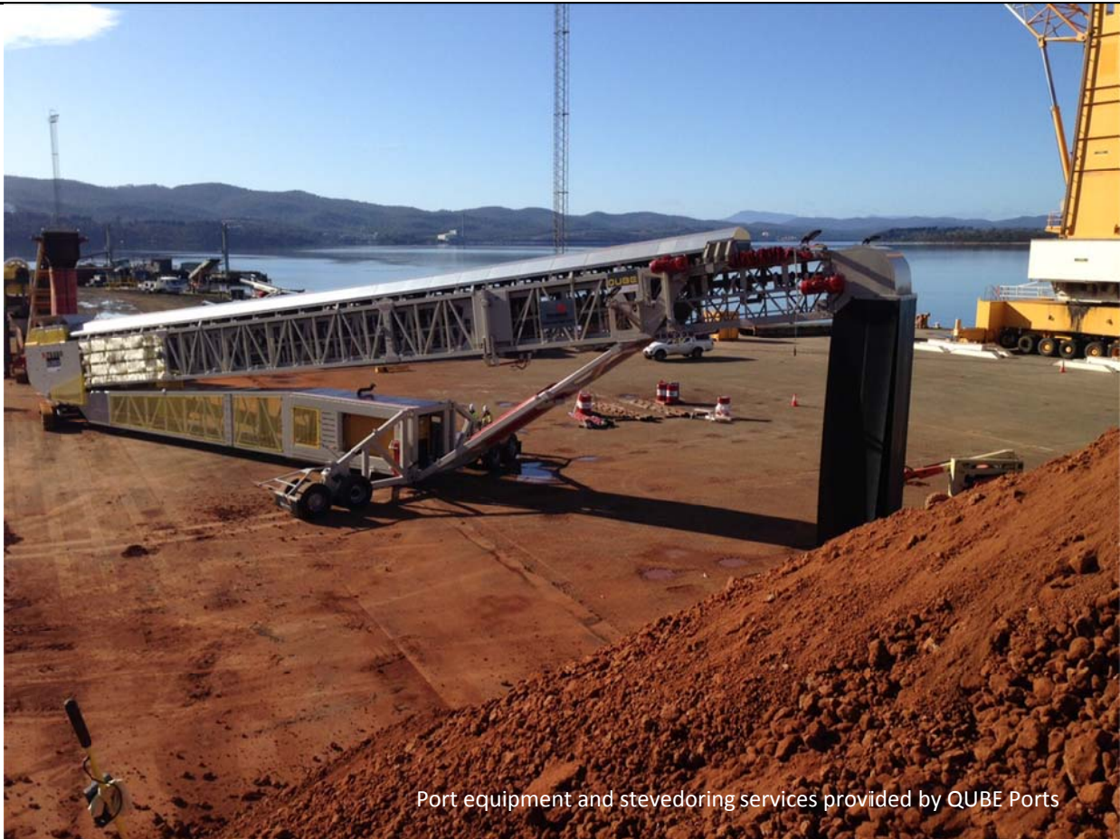
Figure 9: Ship loader has ample air draft height to load the port stockpile at Bell Bay Port to optimum height
