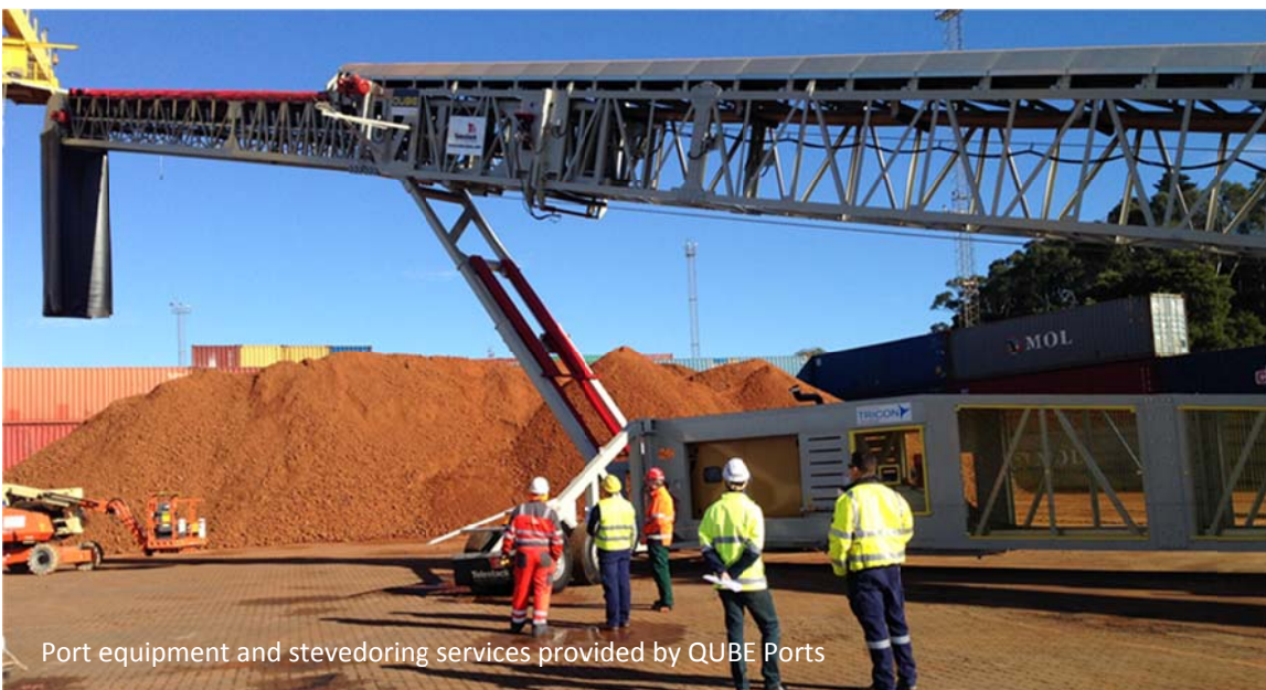
Figure 8: Ship loader used to load onto the port stockpile at Bell Bay Port
