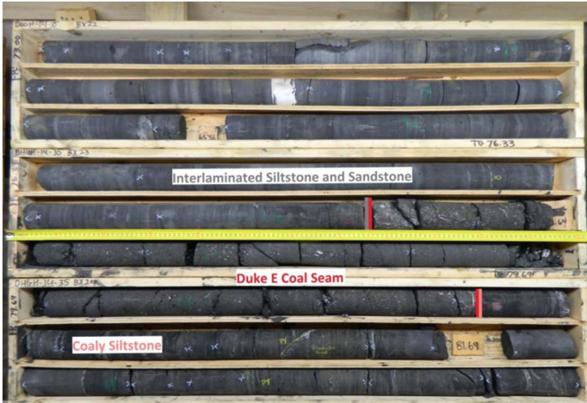
Figure 10: Borehole DDH14-35 (Regional Drilling 2014) Example of core showing flat lying bedding immediately above and below the Duke E Seam
