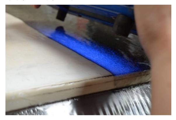
Figure 4 - Scheelite under UV, coming off the wet table.
