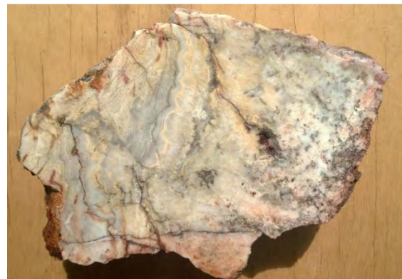
Plate 2c: Colloform banded textures. Pink bands are possibly adularia. Sample assays 230ppb gold, <5ppm arsenic and <1ppm molybdenum. Photo approx. 15cm wide.
