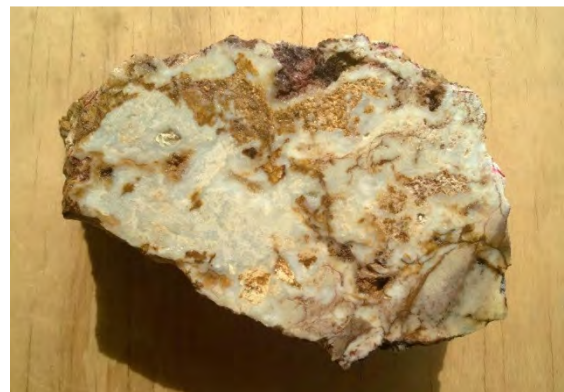
Plate 2b: Very fine grained chalcedonic or agate silica. Sample assays 60ppb gold, 64ppm arsenic and 70ppm molybdenum. Photo approx. 15cm wide.
