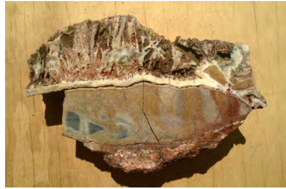
Plate 2a: Bladed silica likely replacing earlier carbonate. Sample assays 10ppb gold, 60ppm arsenic and <1ppm molybdenum. Photo approx. 15cm wide.
