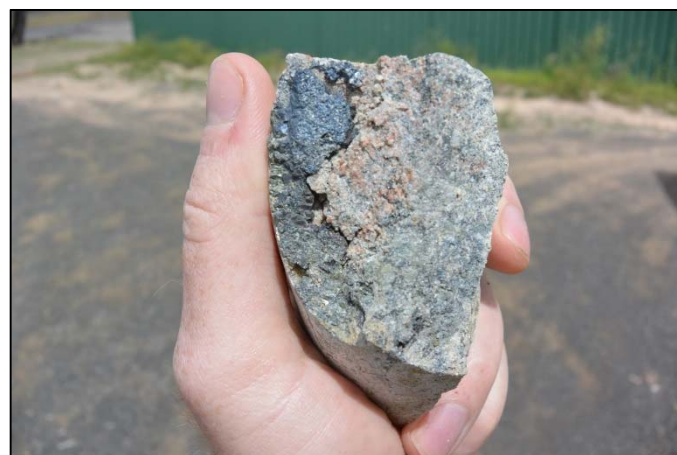
Figure 3. Chalcocite mineralisation within fractures and veinlets of the supergene enriched copper zone.
