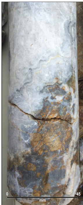
Quartz vein displaying colloform banding. GLD019 drillcore at 11.7 metres.
