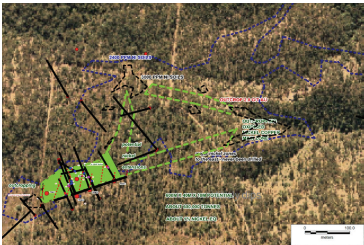
Figure 5: Pembroke drilling locations and interpreted extent of mineralisation
