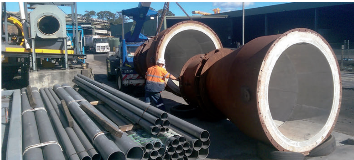
Delivering two fluid bed roaster bodies to be used for gasification in the NZIRP
