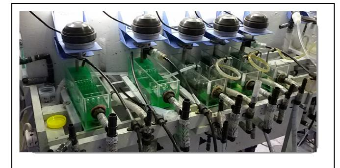
Bench scale CMN process for direct solvent extraction.
