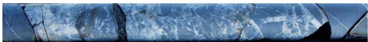
Figure 5. YRDH005 60.5-61m Brecciated slate with calcite/quartz matrix and black puggy material (after sulphide).
