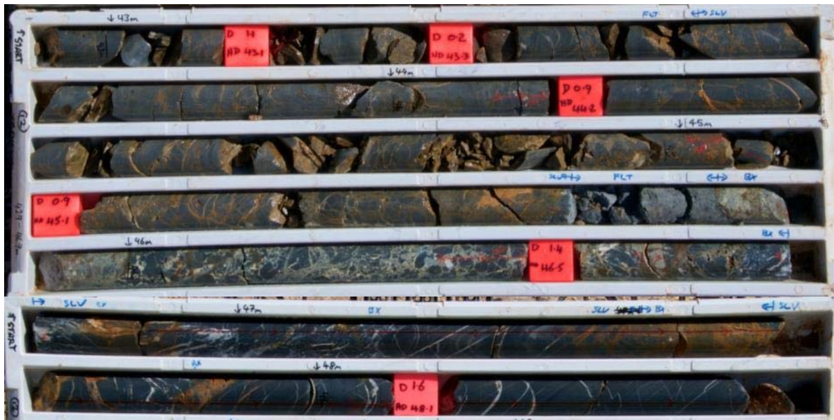
Figure 6. YRDDD005 44.2-48.1 Veining, faulting and brecciation within carbonate rich slate.
