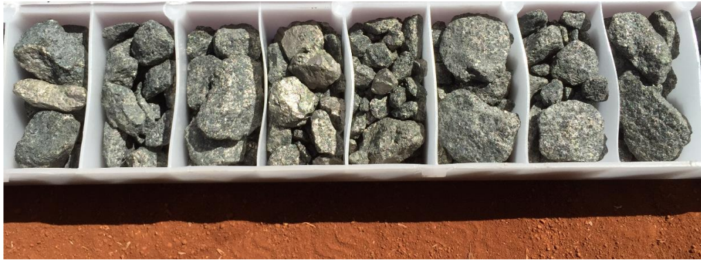
Figure 2. RC chips from the massive and matrix sulphide zone, from 50-58m in hole DMRC0003
