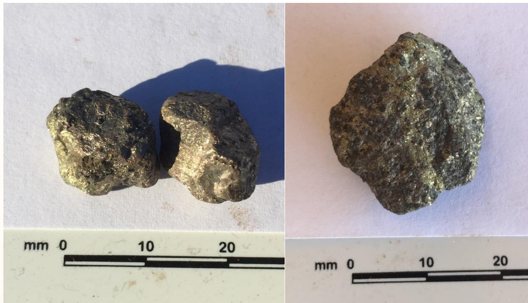
Figure 3. Detailed photo examples of massive sulphide (left) and matrix style sulphides (right) taken from 50-58m downhole drill intercept in DMRC0003
