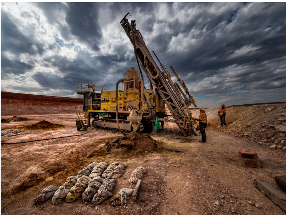
Figure 4 – Thunderbox grade control drilling
