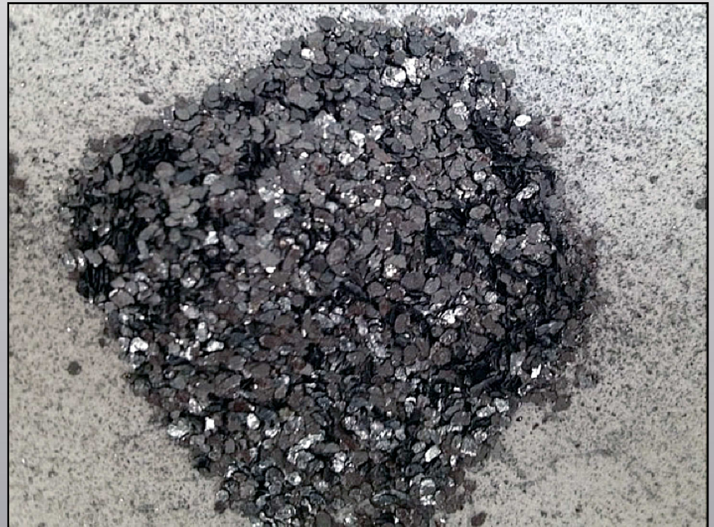
Extra large coarse flakes ( >>600\mu\text{m} ) from diamond core hole (CRD090) at Paxton prospect
