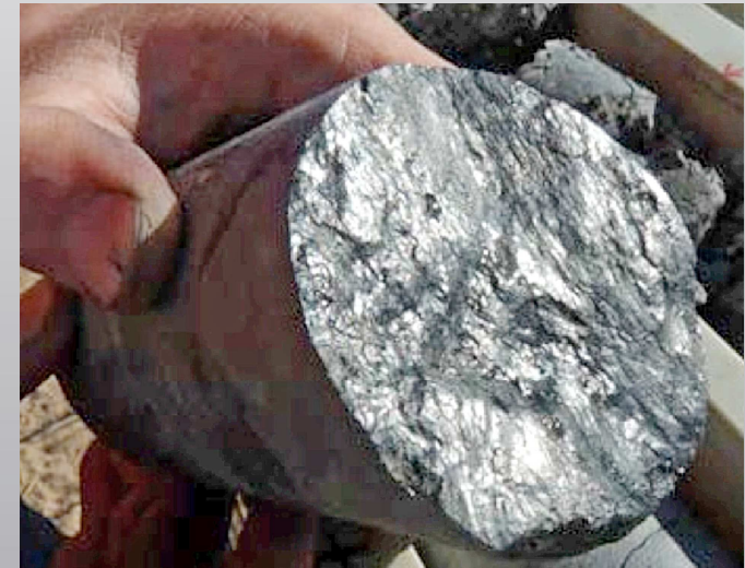
Arno graphite project -- Diamond core drill sample (SIVD007), showing graphitic intersection at Siviour prospect
