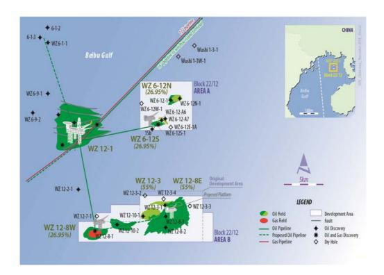
The WZ 12-8W-A6P1 pilot well spudded on 14 November 2015 with the *HYSY931* jack-up rig to evaluate the structural configuration, reservoir quality and oil column thickness in the southeastern part of the WZ 12-10-2 oil accumulation. The well intersected good quality T42 sand close to the oil water contact, defining the southeastern extent of the field (see map below). The horizontal sidetrack was directed updip towards the original discovery location,
