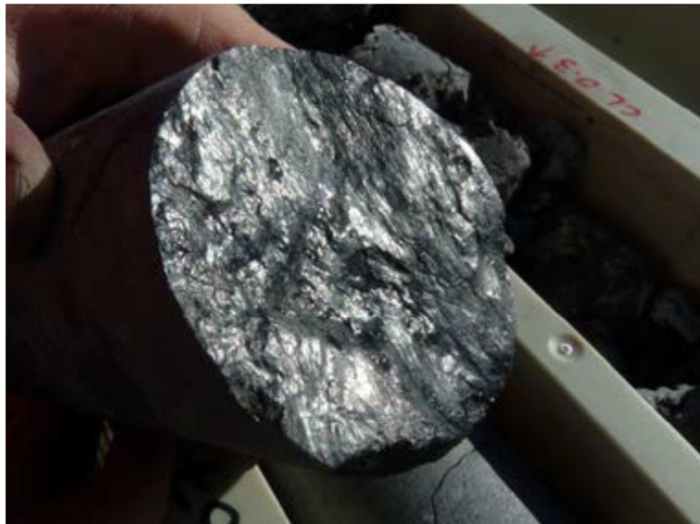
Figure 5. Diamond core drill sample showing graphitic intersection at Siviour prospect (SIVD007, 52.6m to 53.5m @ 9.3% TCG)
