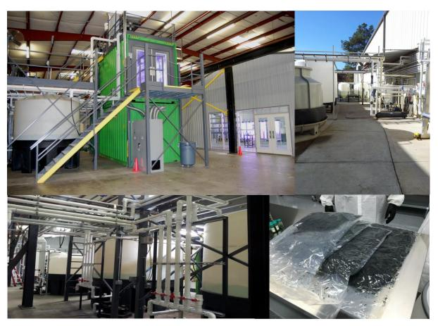
The facility has an output capacity of up to 50 tonnes of algae per year with flexibility to produce and test multiple algal strains based on nutritional requirements. The plant utilises the Company's proprietary enclosed photo-bioreactor technology, which provides a controlled environment for production of high quality algae products for nutraceutical applications. It is expected that the plant will obtain an organic certification within the next few months.
