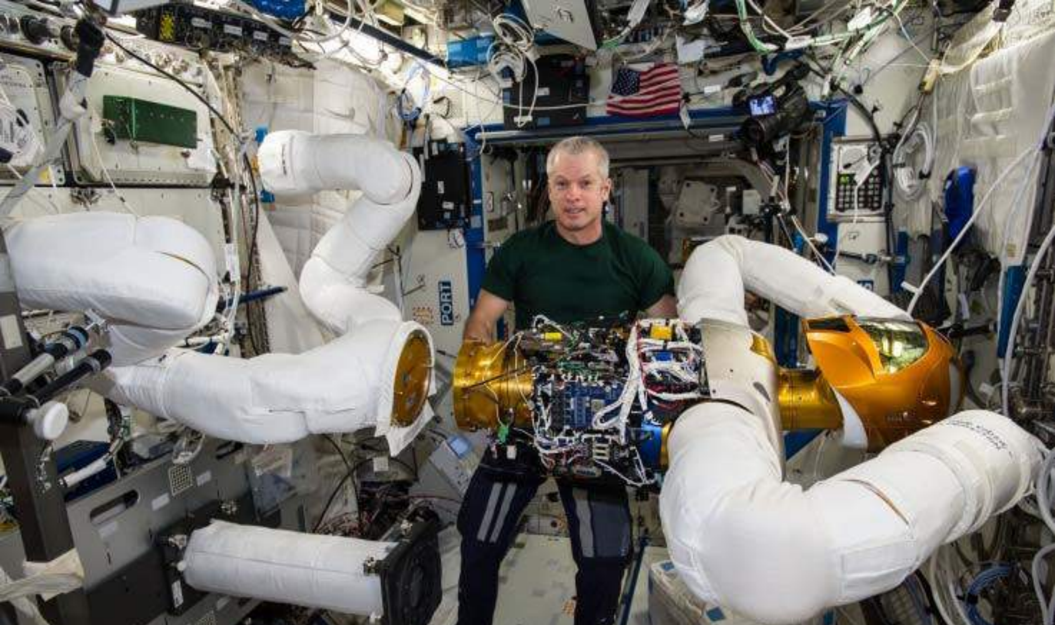
Robonaut 2 delivered February 2011 to ISS. Pictured here with Zero-G leg upgrade which will climb using external handrails.
