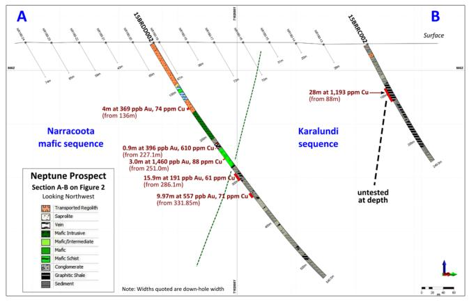
Figure 3: Neptune prospect – Section showing multiple mineralised horizons in 15BRDD002, significant 4m-composite sample results in 15BRRC002, previous RAB/AC drilling and generalised geology.
