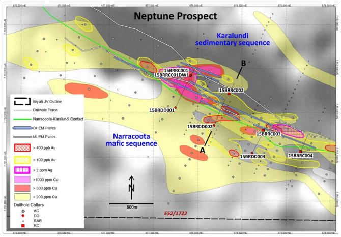
Figure 2: Neptune prospect showing and location of the DD-RC drilling program, previous RAB/AC drilling, geochemical Au-Ag-Cu anomalism, DHEM and MLEM plates over magnetic image.
