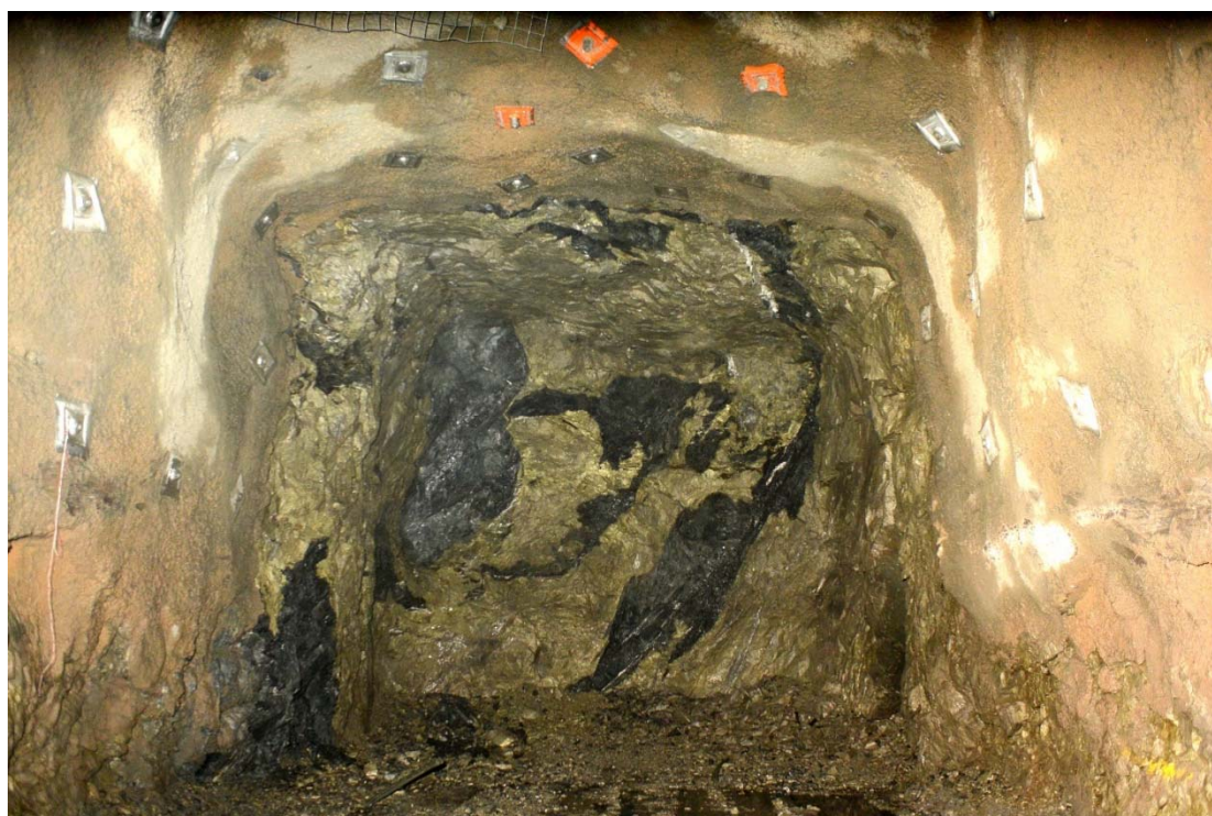
Figure 2: High-grade massive sulphides in the face of a new ore drive in the C5 orebody, January 2016
