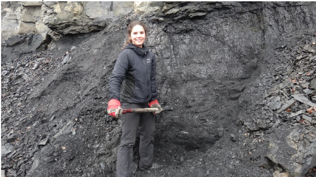
Plate 1. Channel sampling Duke E seam (insitu yields >80% at 10% ash)
