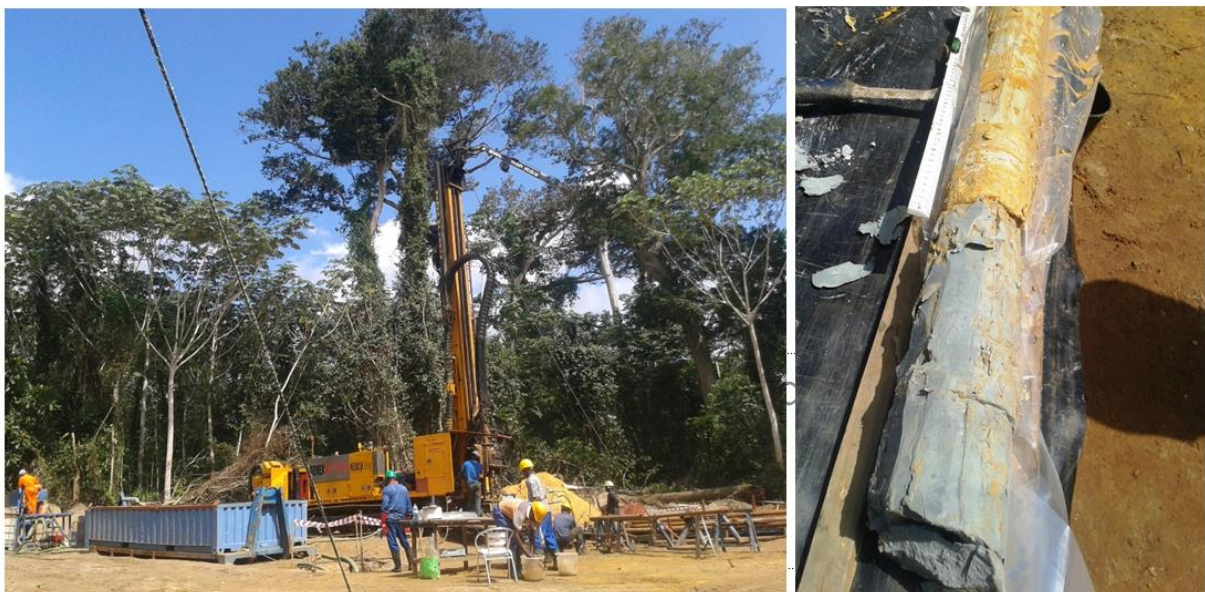
Fig 1. Left; Drilling operations at the Kola Shaft site. Right; Typical core from the Kola shaft site drilling. In this case a clayey siltstone.
