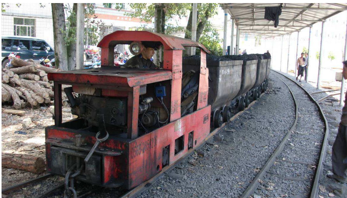
Fig. 5 Locomotive for tub haulage of Caotang Mine
