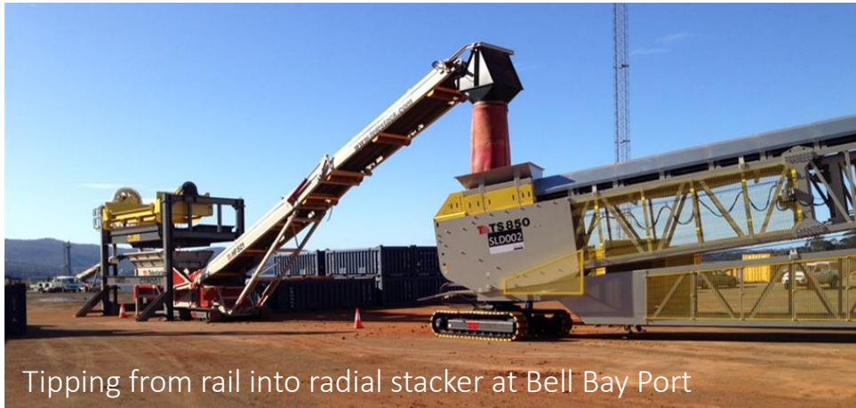
Figure 10: Long-reach radial stacking allows bauxite to be stacked high and peaked to minimise rain penetration and to optimise port area being occupied by the stockpile. Note dust suppression shroud device works well. The bauxite creates relatively low levels of dust, handles perfectly and has a high angle of repose, confirming its excellent handling properties
