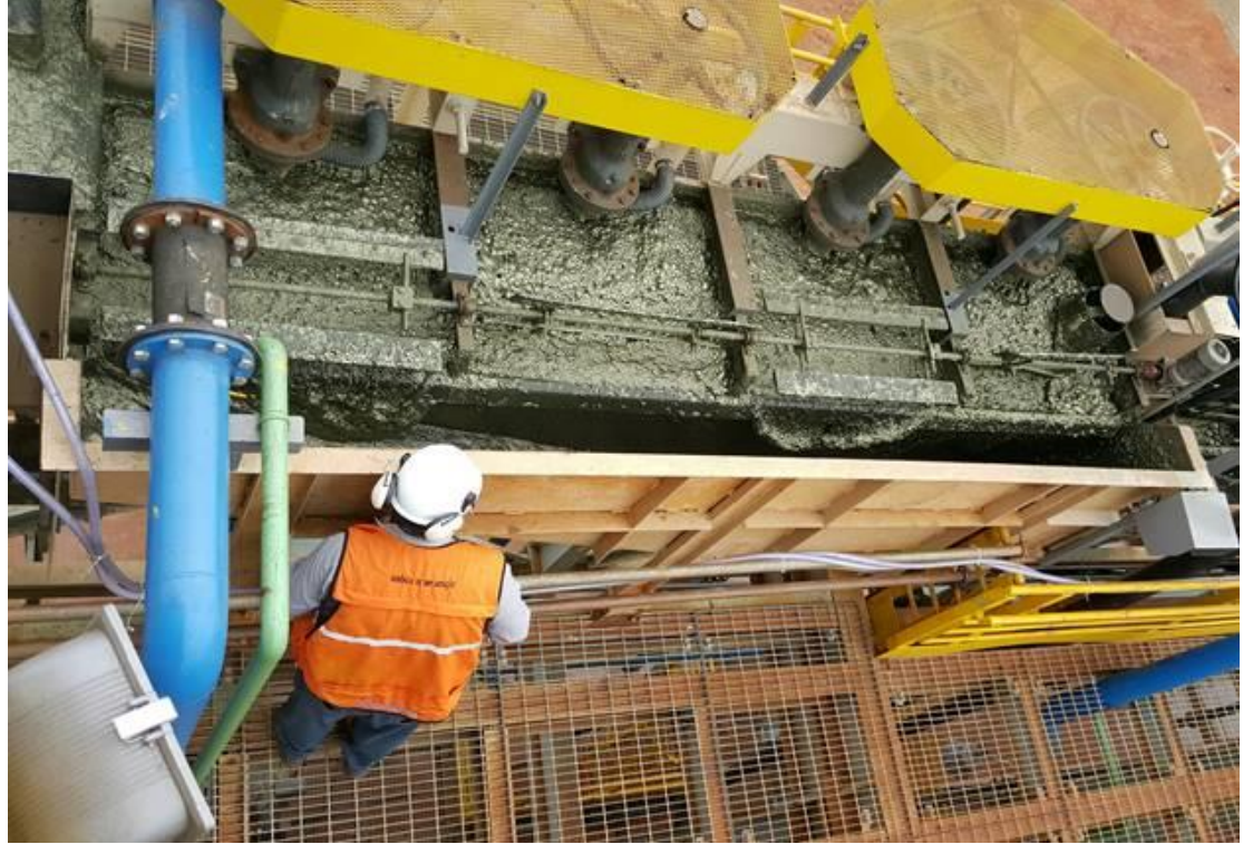
Final flotation copper concentrate assaying ~28% Cu being recovered from the Denver 24 Re-Cleaner cells
