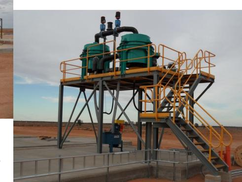
Fully automated dual system Knelson concentrators that can efficiently recover gold over a wide size range, including very fine gold, not included in the current resource.
