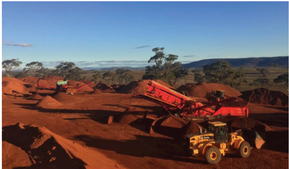
Figure 5: Bald Hill dry screening using “Big Red” and “Li'l Red” screening plants in tandem
