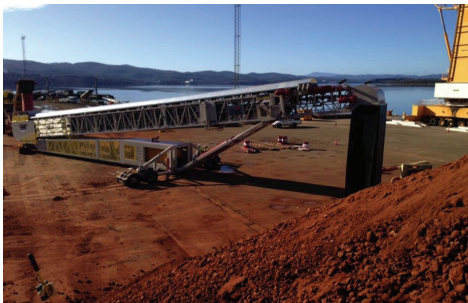
Figure 10: radial stacking to a high peak minimises rain penetration and optimises port area being occupied by the stockpile.
