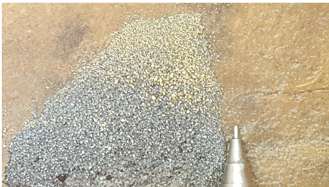
Figure 2: Coarse gold in panned sample from 36-37 metres in hole RCDK016-037 which assayed >100g/t gold
