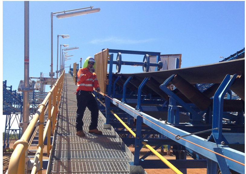
Figure 7: Wet commissioning of Copper Thickener (top image); electrical commissioning activities on the Dust Collector Fan (bottom left), and testing of emergency stop cable on Scrubber Feed Conveyor (bottom right).
