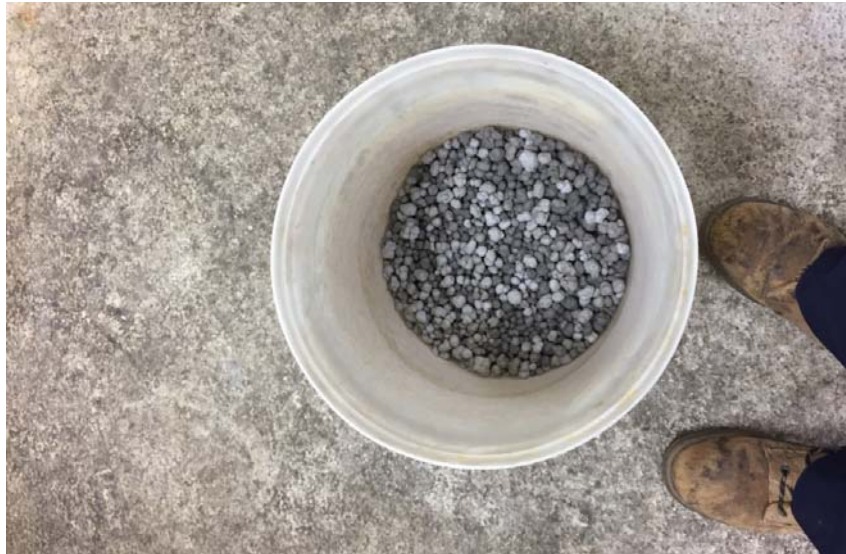
Figure 8: Agglomerates being prepared for testing
