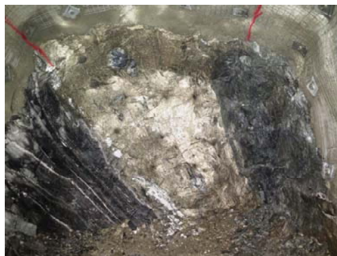
Figure 3: Massive ore in the 200 North ore drive with an average face grade of 6.1% nickel
