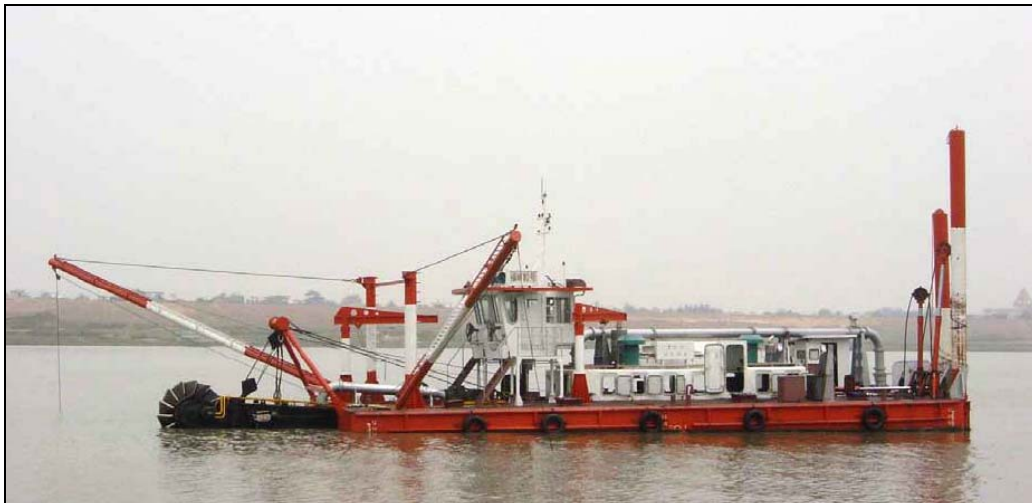
JSSDRI 100m 3 /hr Bucket Wheel Dredge
