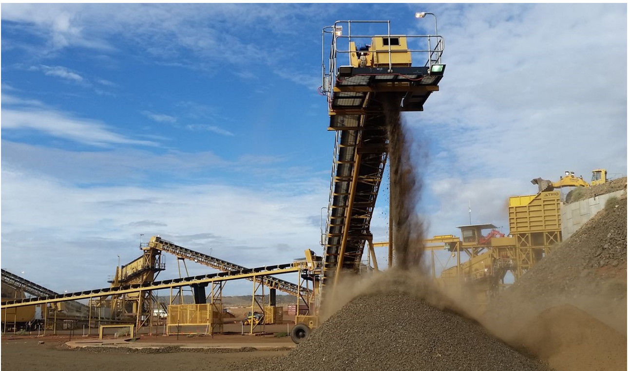
Figure 2: Replacing of the final rolls crusher with a cone crusher resulted from successful test-work using the Company's mobile crushing plant that clearly showed the benefits in separating coarse native copper (+40mm in size), from the associated ore, achieving up to 95% copper concentrate. Top image shows the cone crusher up close and the below image shows commissioning of the cone crusher.
