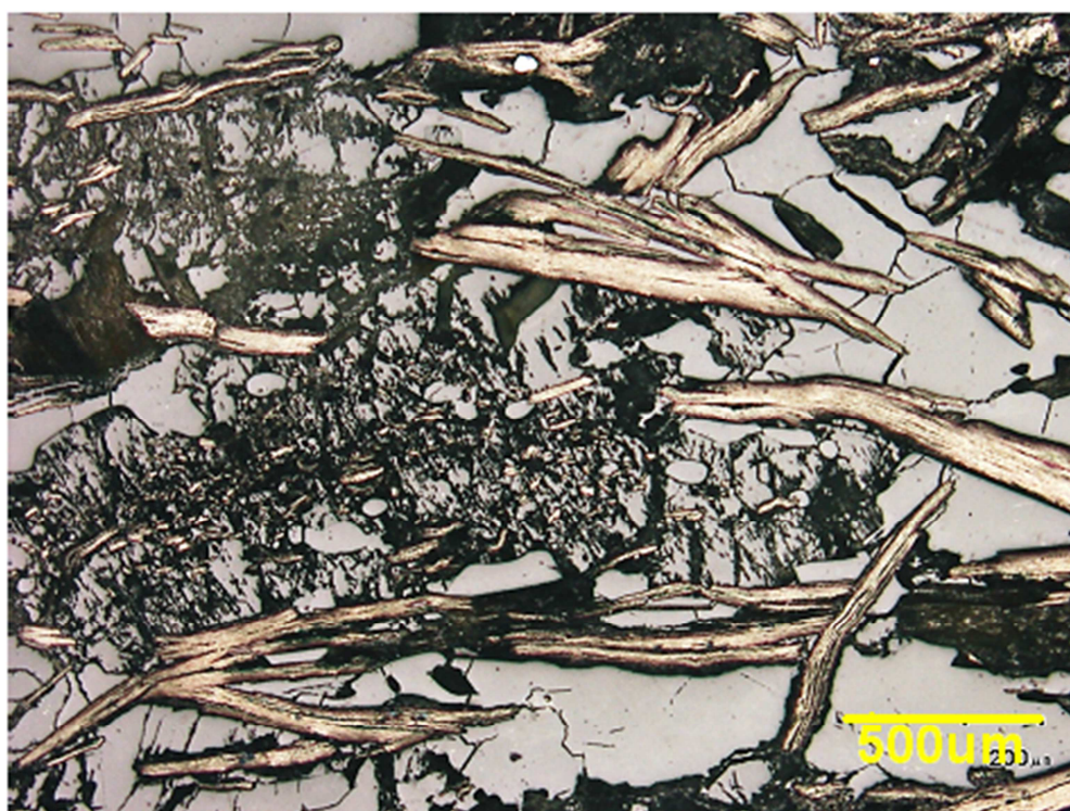
Figure 5. Photomicrograph of graphite flakes from Siv014 (17m to 18m)
