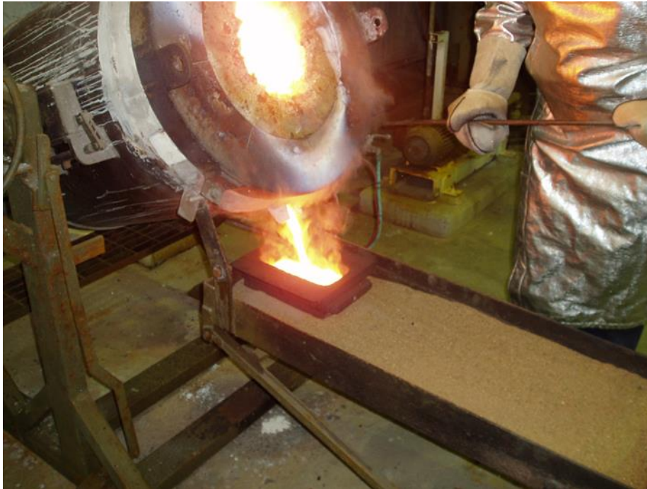
Figure 3. Gold Pour at Maldon Treatment Plant
