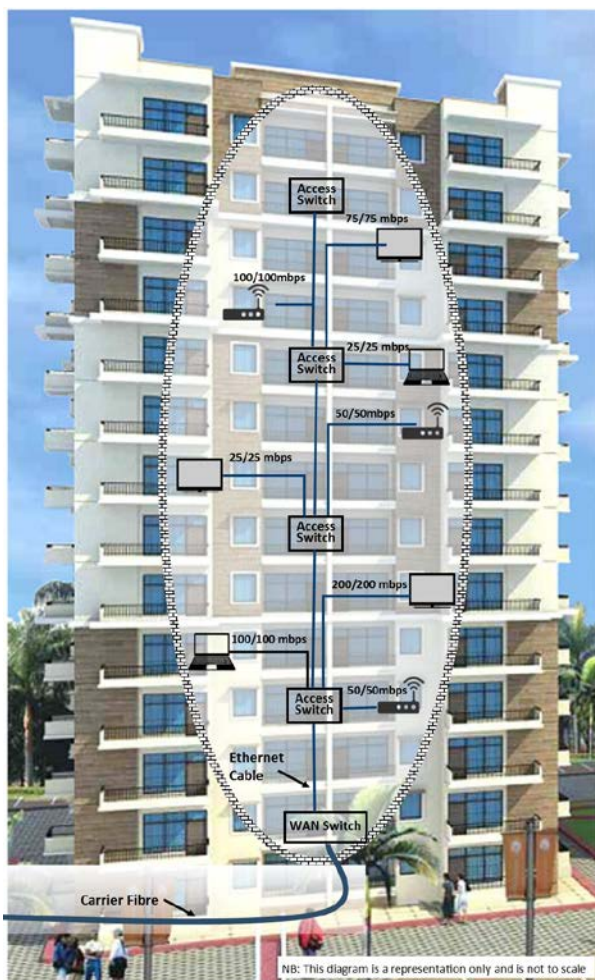
Figure 5 - A typical residential multi-dwelling unit (MDU) deployment
