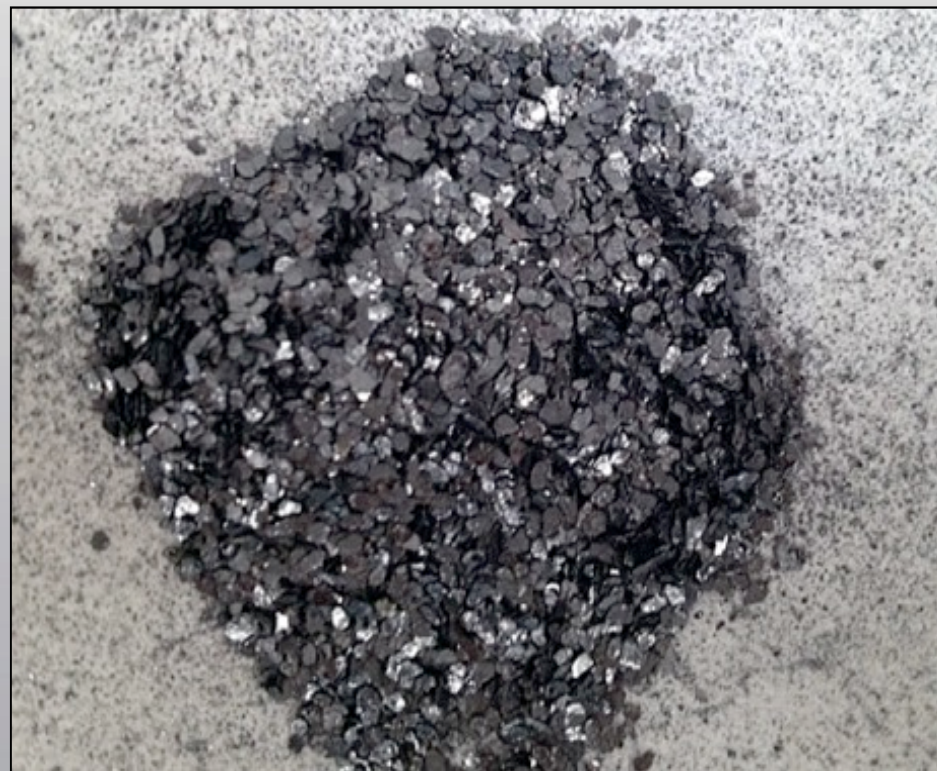
Extra large coarse flakes (>>600 \mu m) from diamond core hole (CRD090) at Siviour prospect
