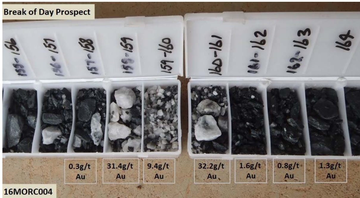
Figure 1: Chip sample tray of RC drill hole 16MORC004 showing quartz vein 158m-161m and individual one metre gold assay results
