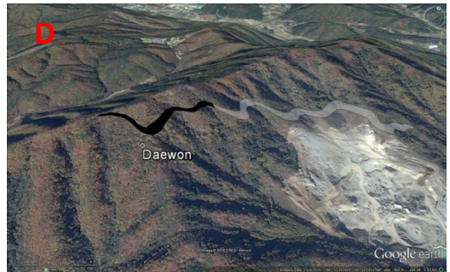
Trace (solid black line) of Graphite Mineralisation as mapped in surface outcrop. Grey shaded area is the interpreted continuation of the structure to the NE. View looking NW in the dip direction.
