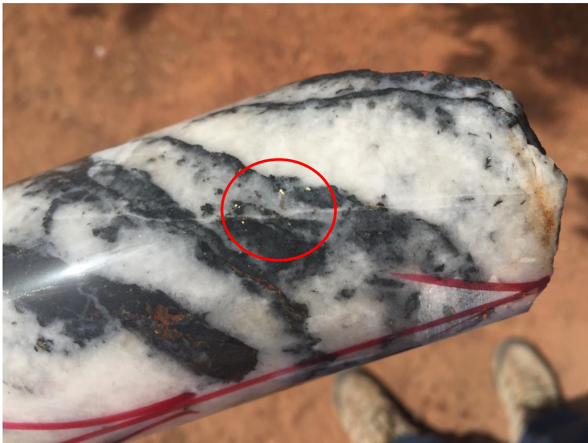
Figure 2: Drill core from DDDK16-002. Later stage quartz vein with visible gold (circled) and fragments of footwall graphitic sediments
