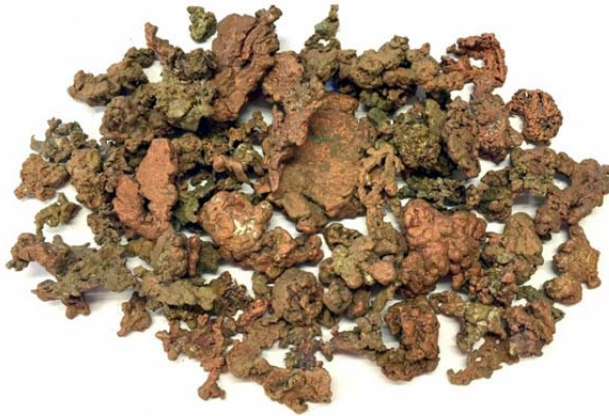
First coarse native copper produced from the Jig circuit
