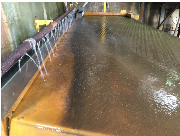
Figures 1A & 1B – Re-commissioning the dressing table with tin concentrate (black stream) on left side of table
