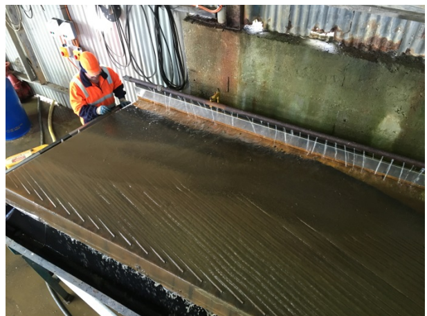
Figures 1A & 1B – Re-commissioning the dressing table with tin concentrate (black stream) on left side of table
