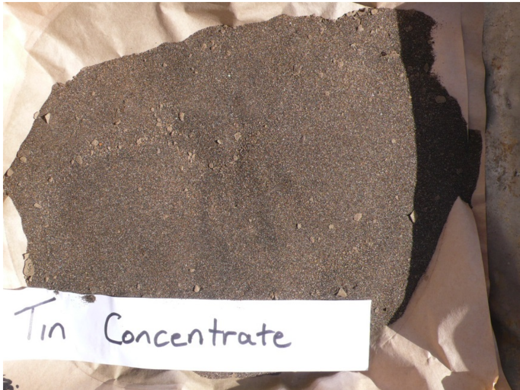
Figure 2 – Sample of final tin concentrate (55% Sn)
