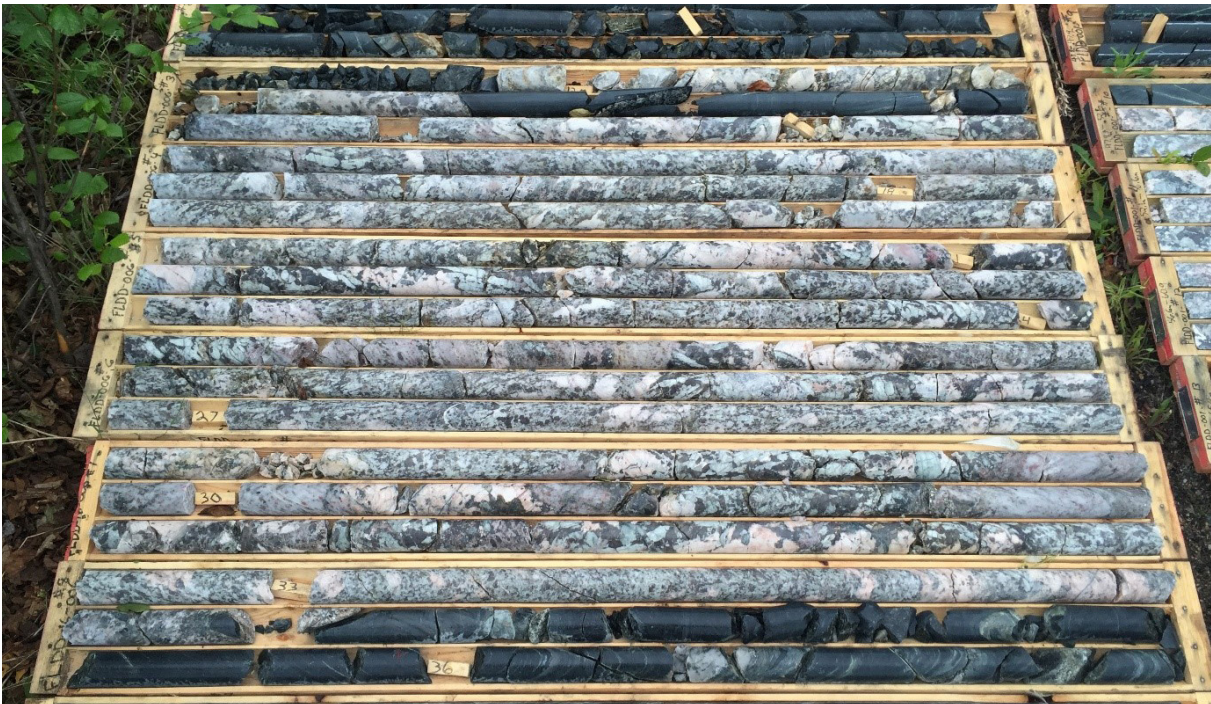
Plate 3 Spodumene bearing pegmatite core from the Falcon Lake West deposit. Core trays 1.5m in length.
