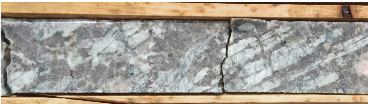
Plate 4 Intense spodumene mineralisation (white mineral oblique to core axis) in Falcon Lake West core.
