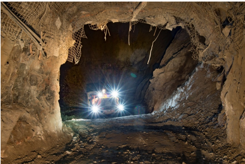
Figure 5 – Karari Underground – Boggging ore from the Dhoni 2140 stope
