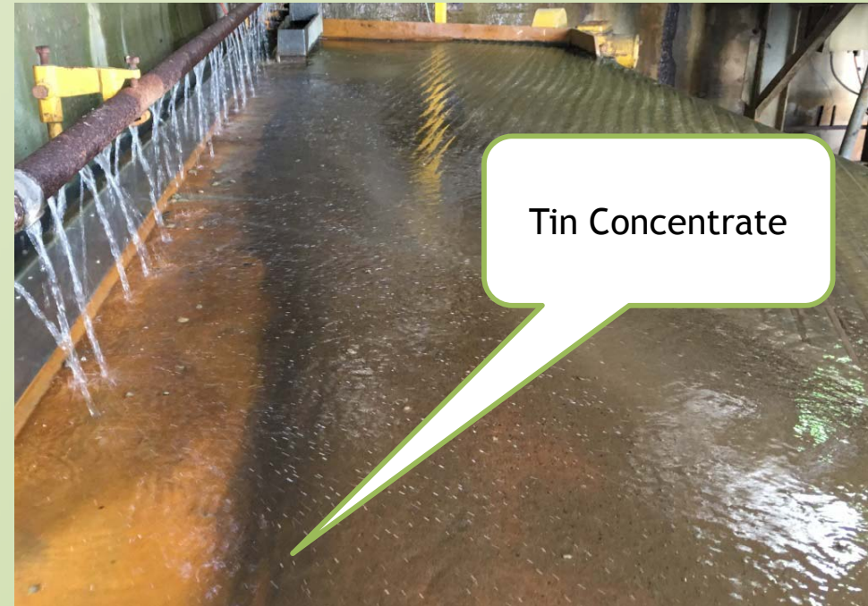
Dressing table being commissioned (tin on left side) 3
