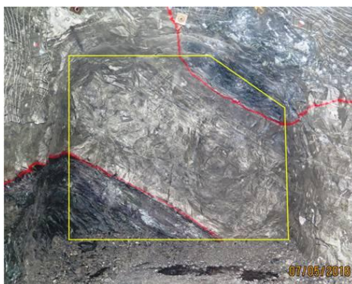
Massive ore at the 862 ore drive (single-boom area) with an average grade of 8.0% nickel
