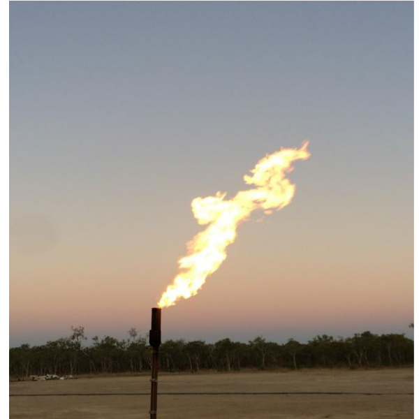
Egilabria-2 well - gas flows from a hydraulically stimulated lateral in shale
